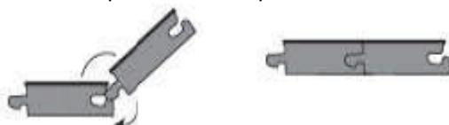
3. Begin the installation of the planks in the left hand corner of the room with the long direction parallel to the incoming sunlight source or to the longest wall of the room (if this is possible). *Be sure to install the first row of boards with the tongue side facing the wall.*
